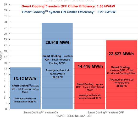
Post-analysis of data monitoring shows **46.8** % improvement in chiller performance achieved by **Smart Cooling™** system during 4 working days.
