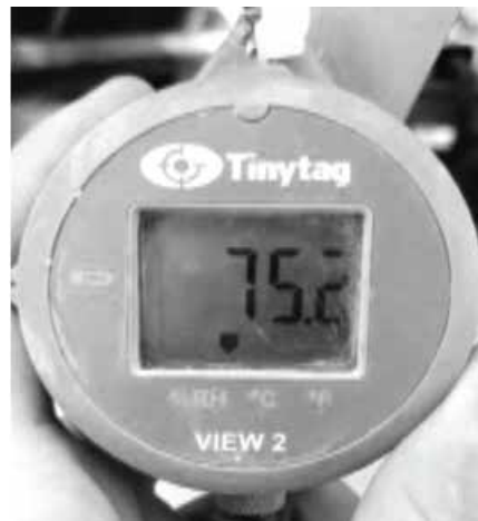
Relative air humidity behind Smart Cooling ™ condenser coil protective membrane RH 75
