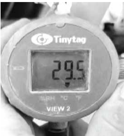
Air temperature behind Smart Cooling ™ condenser coil protective membrane 29 °C
